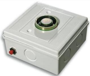
Magnetic hold back devices are used when a fire door is at risk of being propped open (to a kitchen, for example) and you need to make sure it closes if there is a fire. The device is connected to the fire alarm and if activated, the door closes under the action of the self closer.
